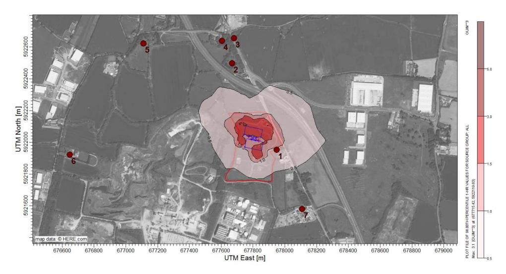
Figure 12-3: Predicted Odour Concentration for the RBSF Component (98 percentile basis)
