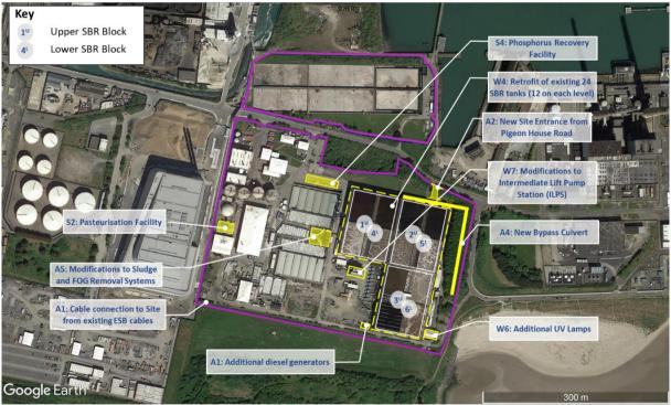
Figure 3-2: Layout of the Proposed Development at Ringsend WwTP
