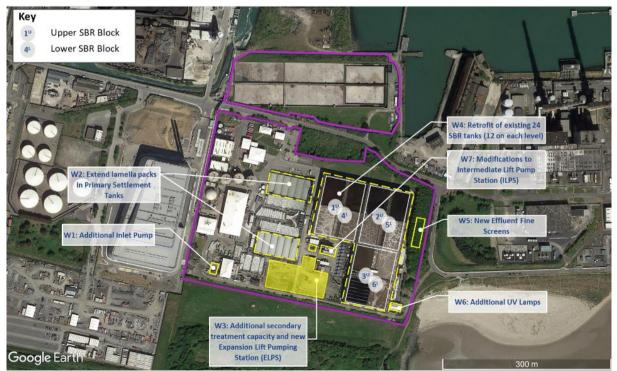
Figure 3-1: 2012 Approval Schematic
