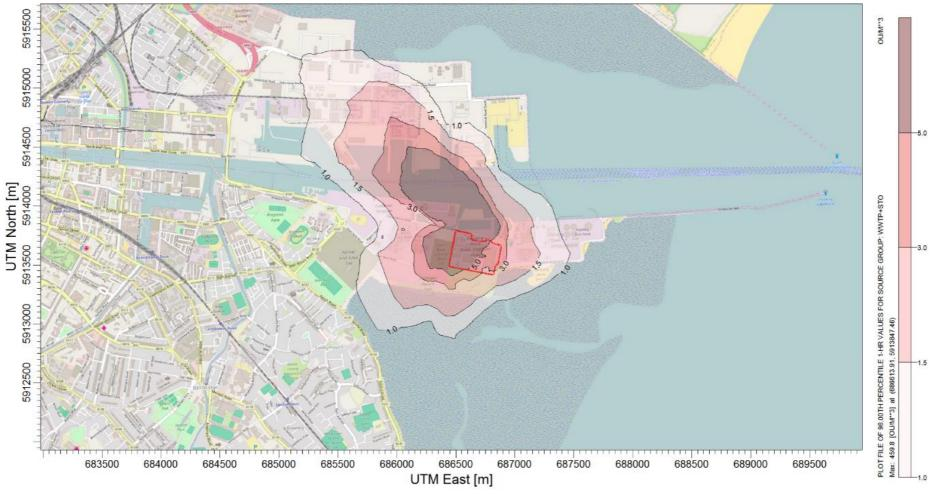
Figure 12-2: Predicted Odour Concentrations for the Ringsend Odour Target (98 percentile basis)
