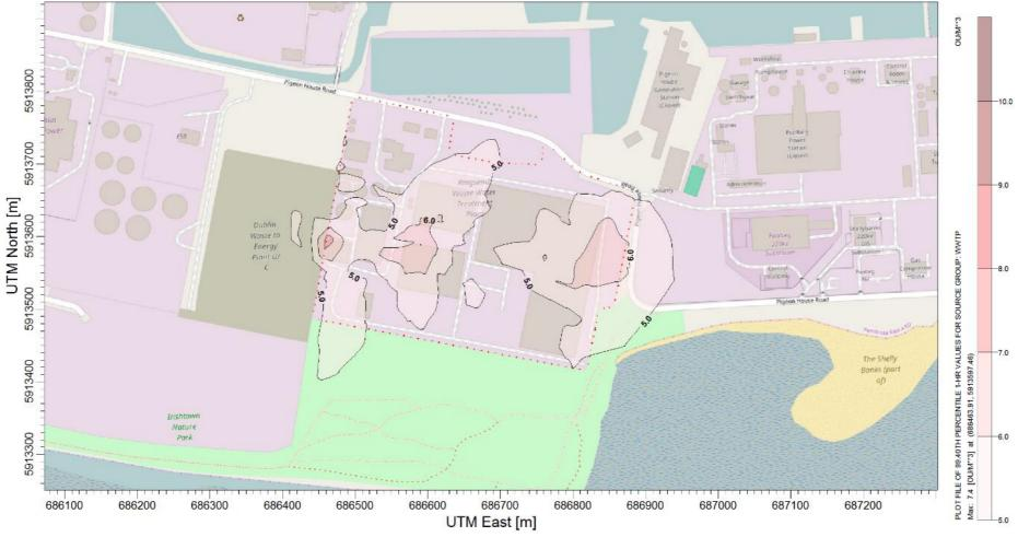
Figure 12-1: Predicted Odour Concentrations for the Ringsend Project Odour Goal Objective (99.4 percentile basis)
